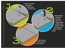
Level Rite Concrete Lifting process is similar to mudjacking, but is an evolved application that allows us to provide our clients with a clean, quick, long-lasting solution. Our process effectively stabilizes soils, fills all voids and lifts concrete using high-density polyurethane foam. The following are the steps for Level Rite Concrete Lifting process:
