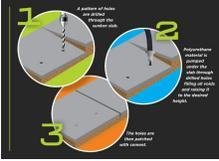
evolved application that allows us to provide our clients with a clean, quick, long-lasting solution. Our process effectively stabilizes soils, fills all voids and lifts concrete using high-density polyurethane foam. The following are the steps for Level Rite Concrete Lifting process:
