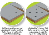
Polyurethane foam is a light weight material compared to traditional mudjacking slurry (2-6 pounds of polyurethane foam vs. 100-130 pounds of mud slurry). Because of the light weight properties of our foam, it won't burden the underlying soils which are often loose and poorly compacted. Mud slurry is extremely heavy and within a couple years can compact the
